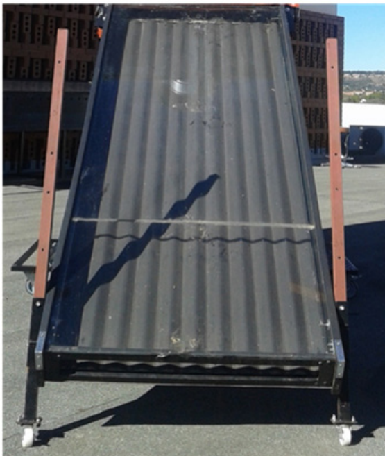
Figure 4: Photo of an air heater.
