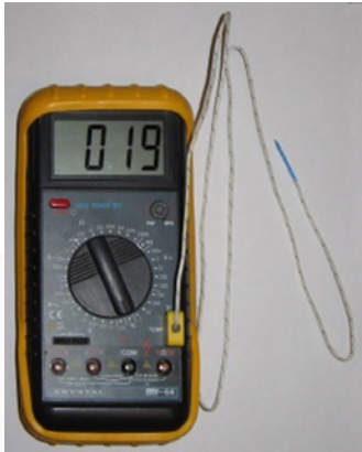
▲ Figure 15: A thermocouple is an electronic thermometer that can be used.
