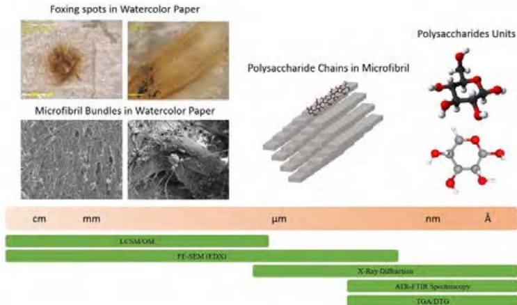
Figure 1. Multi-analytical methods used under various length scales.
