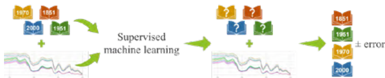
Figure 1. Schematic overview of dating models combining NIR spectroscopic data and machine learning.
