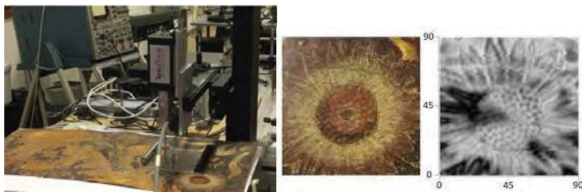
Fig. 1: THz setup operating at 97 GHz in reflection mode. On the right a leather sample and his corresponding reconstructed THz image
