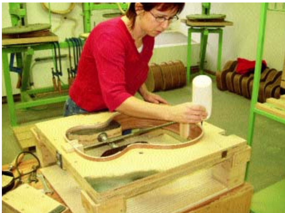
Completing the body of a Furch guitar
