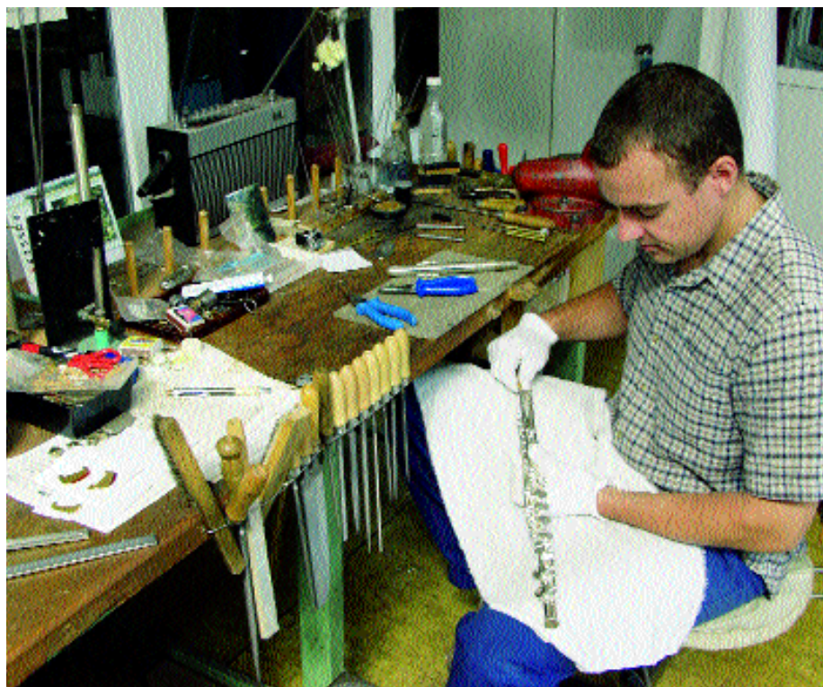
Output control of flutes in the AMATI workshop
