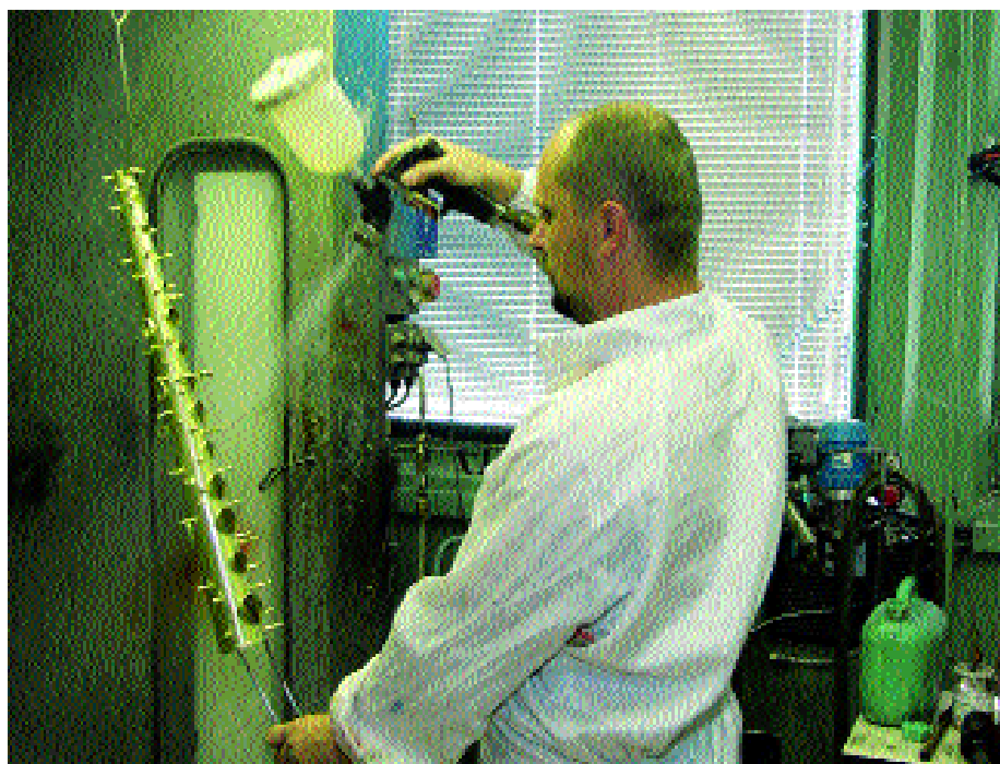
Varnishing the saxophone body
