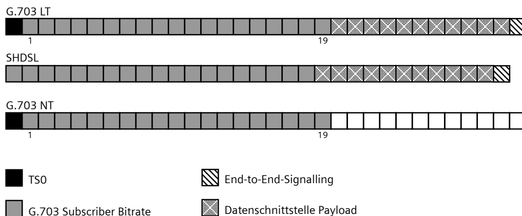
Fig. 1.36 Example 1: SHDSL Mapping with G.703(LT)-'Add/Drop'(NT) mode
