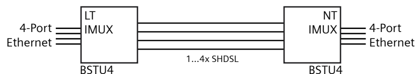
Fig. 1.20 Ethernet / Ethernet mode with BSTU4 – BSTU4
