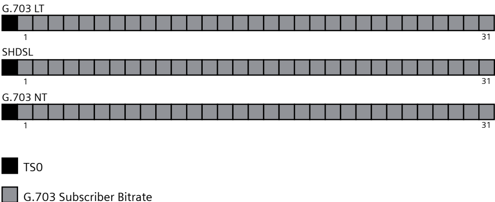
Fig. 1.27 SHDSL Mapping Structured 2 Mbit/s (G.704) and ISDN PRA Mode
