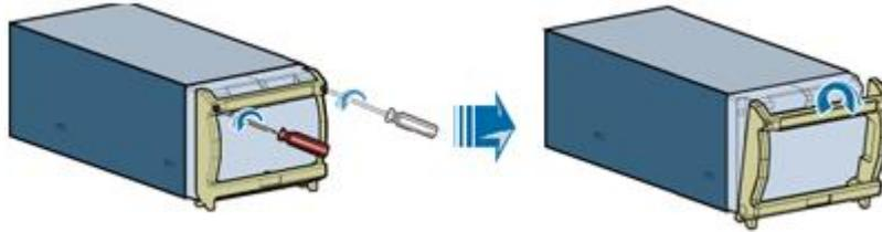
**Figure 5-3** Installing the new rectifier
