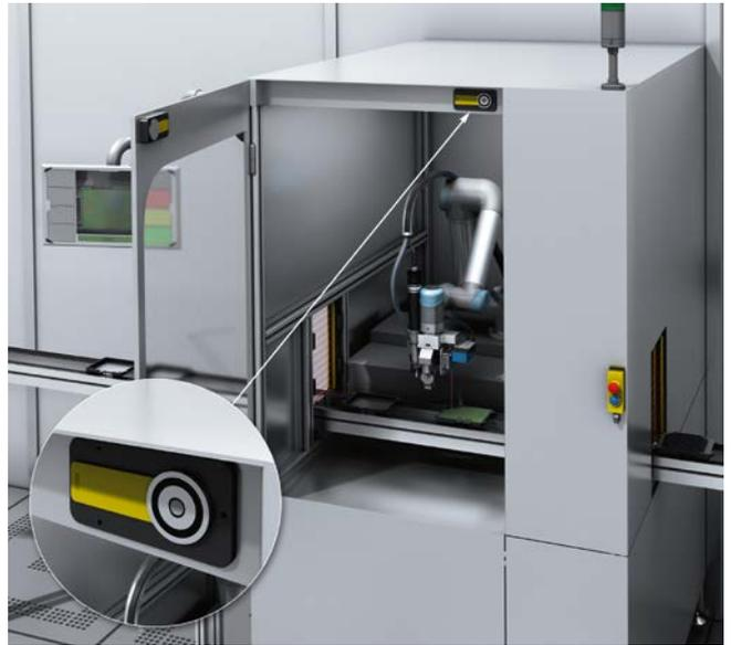
The MLP1 can be integrated almost invisibly into the machine design.
